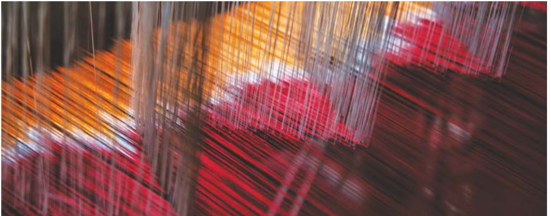
Threads of Tradition: A single Benarasi saree, a symphony of 5600 threads woven into a canvas of 45 inches width. The tale unfurls as perforated cards choreograph their dance, guiding the myriad colored threads to craft a masterpiece that captures the essence of centuries-old artistry, Varanasi
